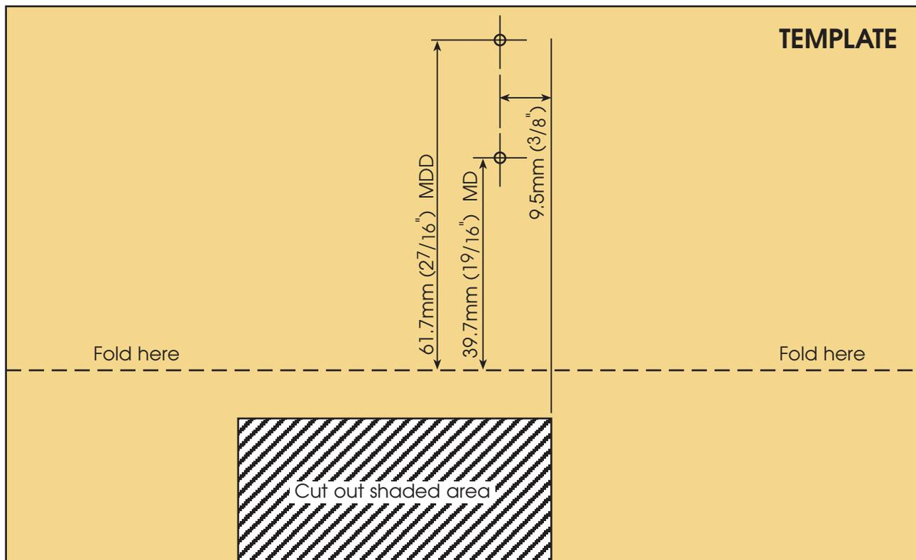
5 Use a **full size** print out of the template, and, if necessary, mount on card. Place the cut-out over the bolt and mark the centre of the keyhole. Turn the template upside down and mark the other keyhole centre.
